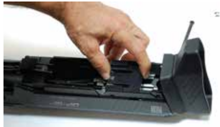
Figure D-10: Slide the retainer plate forward and lift up and out.
