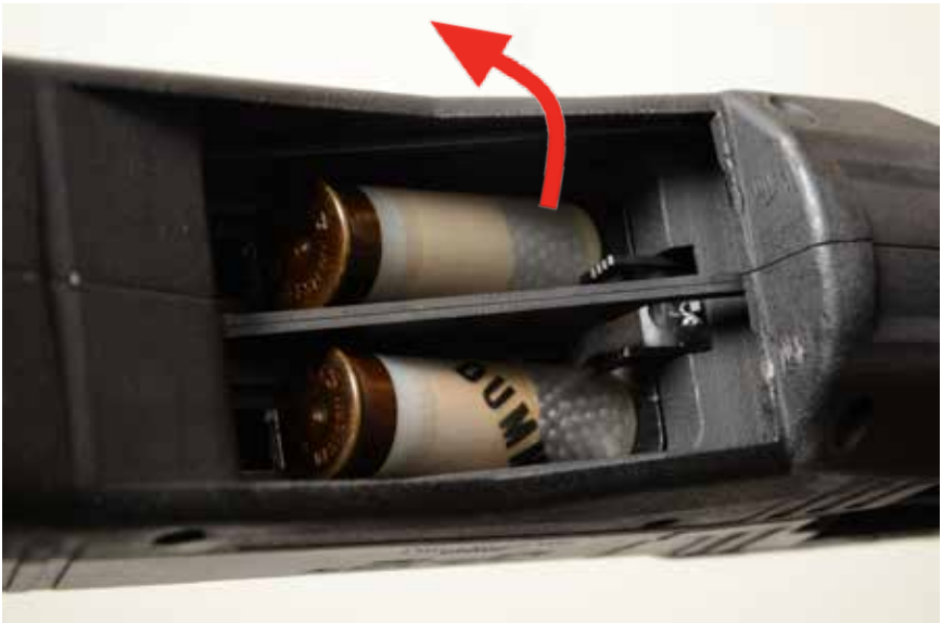
Figure F-1: Clear Double Feed by Rotating Shell Around Lifters
